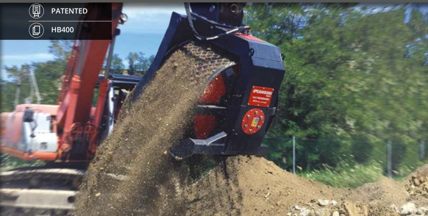
LE NOUVEAU GODET, ET SON NOUVEAU SYSTÈME AVEC DOUBLE PANIER ROTATIF PROJETÉ POUR MACHINES JUSQU'À 35 TONNES, EST ADAPTÉ AUX TRAVAUX DE CRIBLAGE SUR TERRAINS REMUÉS. LA TAILLE DU MATÉRIAU SÉLECTIONNÉ - DE 25 À 65 MM - PEUT ÊTRE VARIÉE DIRECTEMENT ET HYDRAULIQUEMENT DE LA CABINE, SANS REMPLACER AUCUN ÉLÉMENT MÉCANIQUE EN RÉDUISANT LES TEMPS DE TRAVAIL.
