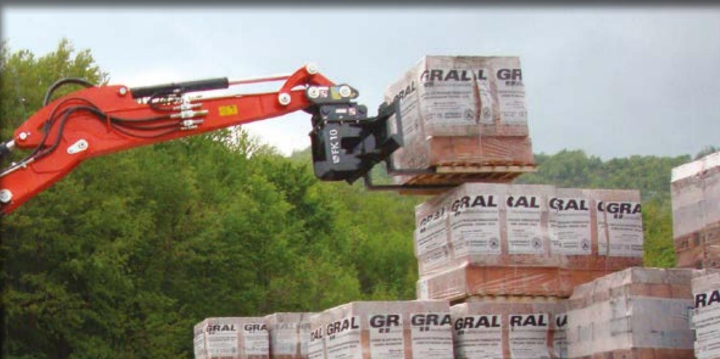
CETTE CONFIGURATION PERMET L'ACCROCHAGE AUX PELLES ET REND LE TABLIER APPROPRIÉ POUR LA MANUTENTION DES CHARGES DANS DE ZONES DURES D'ARRIVER AUTREMENT.
