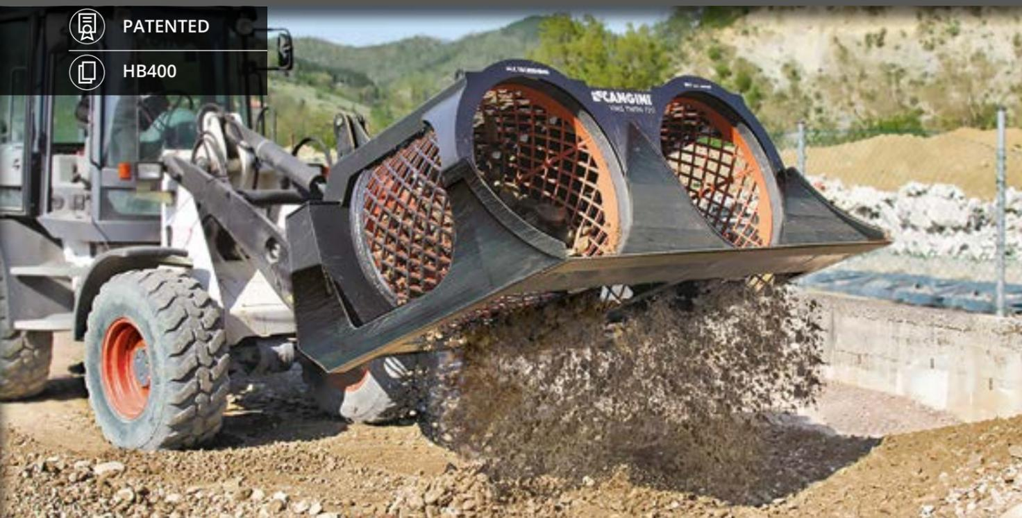
LE NOUVEAU GODET MULTISCREENING DOUBLE, ET SON NOUVEAU SYSTÈME AVEC DEUX DOUBLES PANIERS ROTATIFS JUMELÉS DANS UN SEUL CHÂSSIS, PROJETÉ POUR ACCOUPLEMENT FRONTAL, EST ADAPTÉ AUX TRAVAUX DE CRIBLAGE SUR TERRAINS RÉMUEÉS. LA TAILLE DU MATÉRIAU SÉLECTIONNÉ - DE 25 À 65MM - PEUT ÊTRE VARIÉE DIRECTEMENT ET HYDRAULIQUEMENT DE LA CABINE, SANS REMPLACER AUCUN ÉLÉMENT MÉCANIQUE EN RÉDUISANT LES TEMPS DE TRAVAIL.
