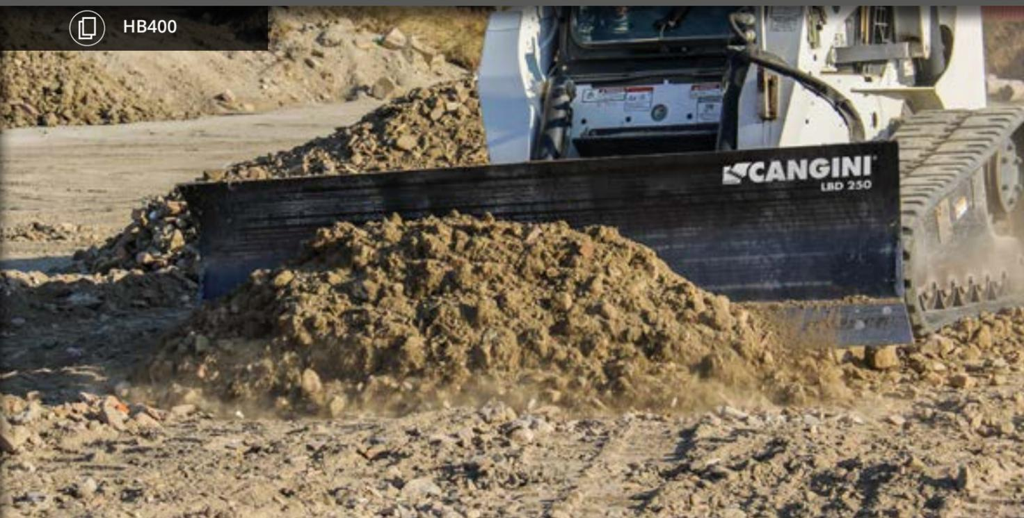
LA LAME DE BULL EST CONÇUE POUR DES TRAVAUX COMME LE NIVELLEMENT DES TERRAINS ET L'ÉTALEMENT DE MATÉRIAUX RAPPORTÉS. LA STRUCTURE EXTRÊMEMENT ROBUSTE EST IDÉALE POUR RÉSISTER AUX SOLLICITATIONS LES PLUS ÉLEVÉES. DOTÉE AUSSI D'UN SYSTÈME D'INCLINAISON PAR RAPPORT AU PLAN HORIZONTAL NOMMÉ TILT ET D'INCLINAISON LATÉRALE NOMMÉ ANGLE. SUR LE VERSOIR, DEUX PATINS PERMETTENT DE RÉGLER L'ENFONCEMENT DE LA LAME DANS LE TERRAIN.
